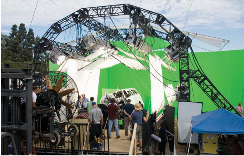
An elaborate rig Nolan wryly dubbed "the tunnel of expense" was constructed from truss to capture a shot of a van rotating 360 degrees on its horizontal axis.
