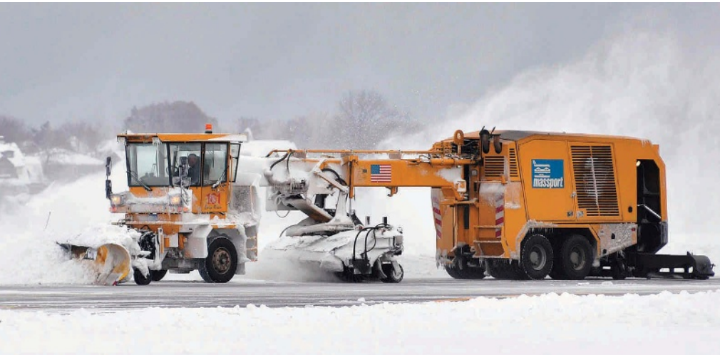
Snow removal equipment at Logan are equipped with GPS transmitters to track location and performance. Photo Credit: Rudy Chiarello, Massport.
