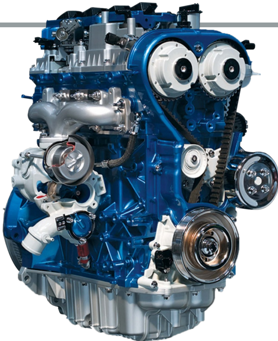
The 1.6-L EcoBoost is based on Ford's Sigma family architecture. The twin independent cam phasers each operate in conjunction with one oil-control solenoid per camshaft. Note cast exhaust manifold, structural oil pan, BorgWarner low-inertia KP39 turbocharger.
