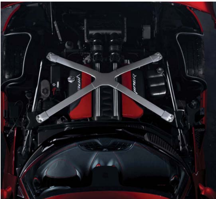
Underhood of the 2013 Viper is an 8.4-L aluminum V10 engine and an aluminum x-brace for stiffness. Torsional rigidity by 50% compared to the old car, Gilles reported.
