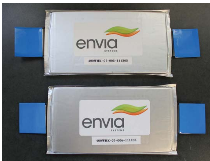
Envia System chose a pouch design for its cell. Shown are samples of the company's new high-energy-density, 45-A·h lithium-ion cells.
