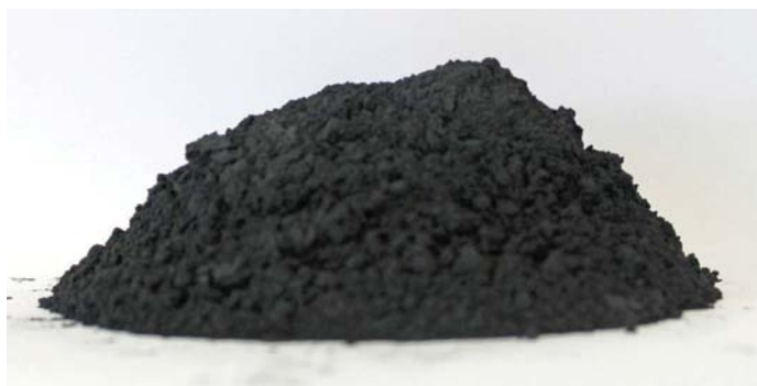
Envia's high capacity manganese-rich cathode material is stable at high voltages and handles high charge fluxes in long-term use.
