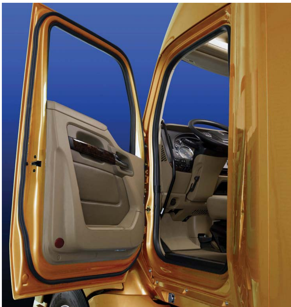
One factor heavy-truck interior designers must consider that their automotive counterparts do not is under-dash finishing pieces. Also shown is the triple-sealed, stamped aluminum door of the Kenworth T680, which contributes to a 40% reduction of interior noise in the new truck.
