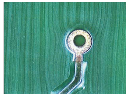
FIGURE 3. Selective added solder layer over conductor and holes free of solder by digital ink-jet printing technology.
