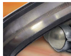
Fluted race caused by VFD-induced discharges through the bearings of unprotected motor. AEGIS™ SGR prevents such damage.
