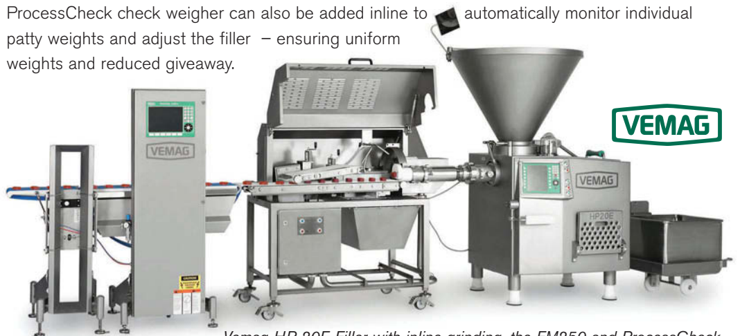
Vemag HP 20E Filler with inline grinding, the FM250 and ProcessCheck
