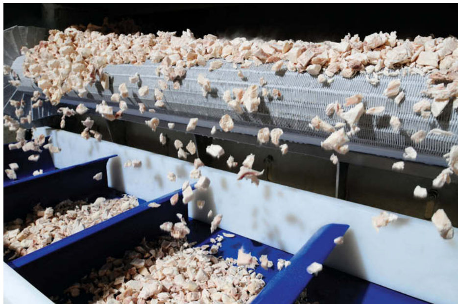
Linde's Cryoline Cryowave IQF freezer features rolling-wave action designed to prevent products from clumping together or sticking to belts.
