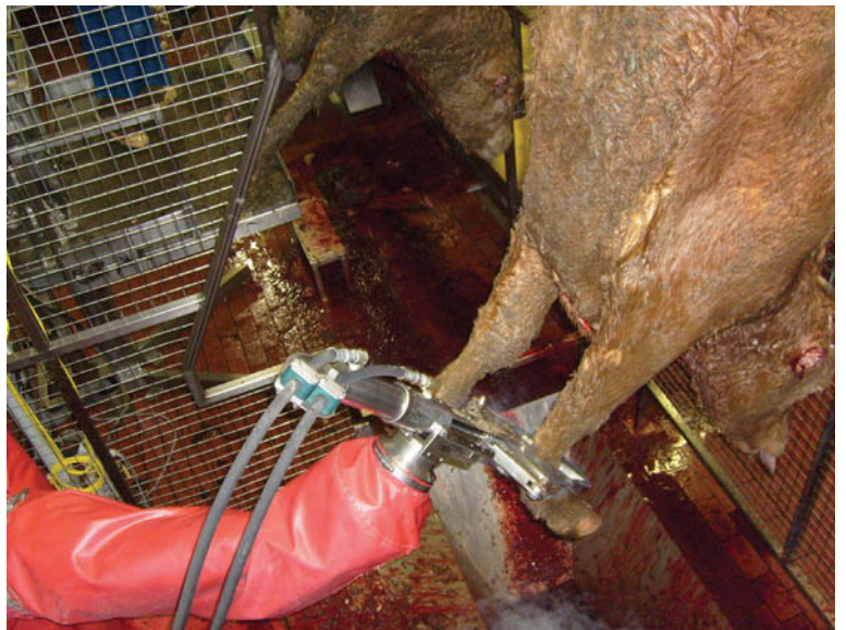
Model JR-50 Hock Cutter Robot with Jarvis' 30CL-1R Hock Cutter
