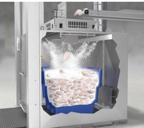
Praxair's Even Chill system uses carbon dioxide snow supplied via a PLC-controlled injection system.
